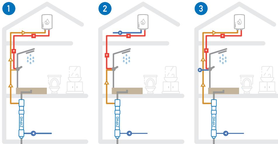
The preheated water is transferred to the tap and the boiler - the most efficient configuration.
